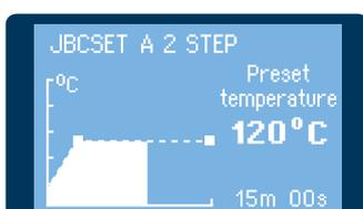
The control Thermocouple follows a temperature profile precisely and with the auxiliary thermocouple the PCB's components will be protected.
